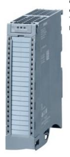
SIMATIC S7-1500, Analog input module AI 8xU/R/RTD/TC HF, 16 bit resolution, up to 21 bit Resolution at RT and TC, Accuracy 0.1%, 8 channels in groups of 1, Common mode voltage: 30V AC/60V DC, diagnostics; Hardware interrupts scalable Temperature range, Thermocouple type C: Calibrate in RUN incl. infeed element, Shield bracket and shield terminal
