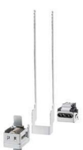
SIMATIC S7-1500, spare part Shielding set Consisting of: \* Shield clamp, \* Shield bracket, \* 24 V DC infeed element in Screw-type connection system, suitable for analog and technology modules of the S7-1500 suitable for all front connectors for 35 mm wide modules 5 units per packing unit
