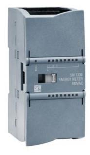
SIMATIC S7-1200, Analog input, SM 1238 Energy Meter 480 V AC, power measurement module for data acquisition in 1- and 3-phase supply systems (TN, TT) up to 480 V AC; Current range: 1 A, 5A; acquisition of voltage, current, phase angles, power, energy values, frequencies; Channel diagnostics
