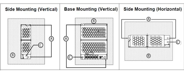
Fig. 2 Mounting Orientation
