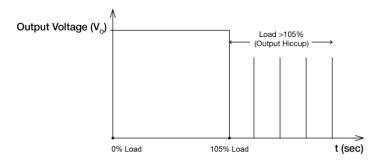
It is not recommended to prolong the duration of Io when it is <105% but >100%, since it may cause damage to the PSU.
