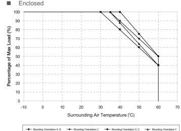
Fig.1.2 De-rating for Mounting Orientation A, B > 40°C de-rate power by 2.5% / °C
