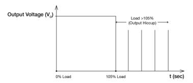
Additionally, if the  $I_0$  is <105% but >100% for a prolong period of time (depending on the load), the Over Temperature Protection (OTP) will be activated due to high temperature on critical components. The power supply will then go into latch mode until the fault is removed and the mains is reapplied.
