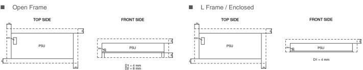
For safety reasons, please ensure the mounted device is kept at  $\geq$  4mm (0.16 inch) safety distance at all sides from other components and equipments. Please insert an insulation sheet between the system and product, if the safety distance is less than 4mm (0.16 inch).
