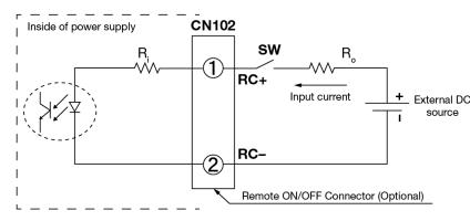
You can remotely control the power supply unit to turn ON/OFF by using an external DC source. Follow the DC power source voltage and current limiting defined in the table below.
