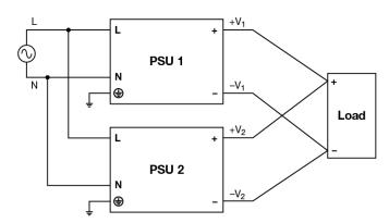
Fig. 4 Parallel Operation Connection Diagram
