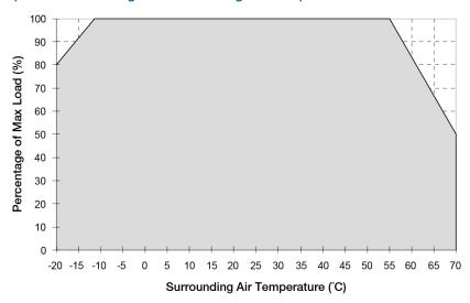
Fig. 1 De-rating for Vertical Mounting Orientation
