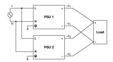
Fig. 4 Parallel Operation Connection Diagram
