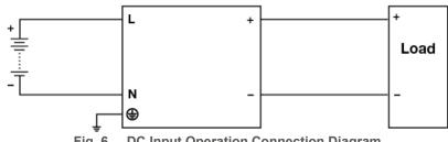
**DC Input Operation Connection Diagram** Fig. 6
