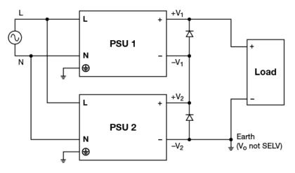
Fig. 5 Series Operation Connection Diagram
