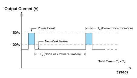
Fig. 7 Duty Cycle Calculation
