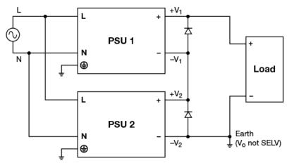
Fig. 11 Series Operation Connection Diagram
