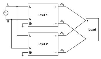
Fig. 10 Parallel Operation Connection Diagram
